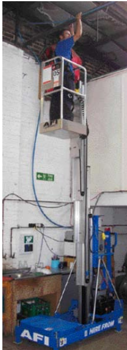
■ Above: AFI's new Genie IWP20s have ultra narrow platforms for access into the tightest of places.
