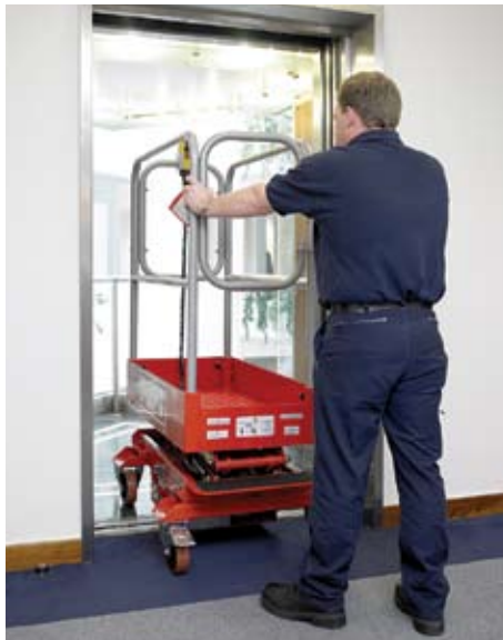
The Leonardo Bravi weighs only 450kg, making it ideal for working on floors where point loading is an issue. The Leonardo has a working height of 4.90m, an extended platform length of 0.68m by 1.71m, and can turn within its own axis, making it extremely manoeuvrable.
