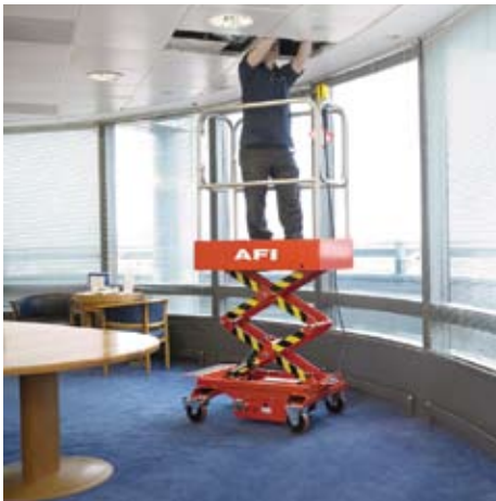
Above and right: AFI's fleet of Pop-Up machines have a working height of 3.63 metres, a closed height of only 1.64m and a width of just 0.70m.
