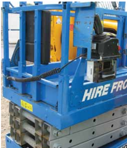
The Infobric unit on a scissor lift.
